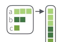
**flatten(x)** Remove a level of indexes from a list. Also **flatten\_chr**, **flatten\_dbl**, **flatten\_dfc**, **flatten\_dfr**, **flatten\_int**, **flatten\_lgl**. **flatten(x)**
